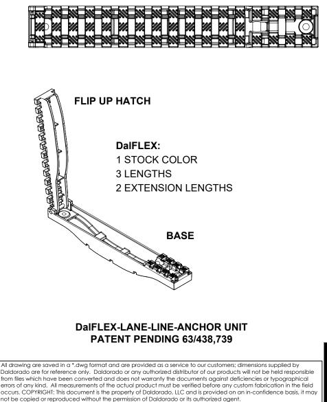
**DaIFLEX:** A LANE LINE ANCHOR UNIT THAT IS NON CORROSIVE AND DOES NOT REQUIRE BONDING. THE UNIT IS FORMED OF TWO MOLDED PVC SECTIONS CERTIFIED ANSI/NSF/CAN 50-2020 SECTION 22.3 AND A LANE LINE EXTENSION.
